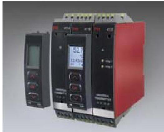
The PR electronics model 4116 DIN rail mounted single oxygen transmitter will accept an input directly from our Oxygen Probes. If you want to display and alarm for both oxygen and temperature (PT100 sensors) then two transmitters will be required. The transmitter can then send the value back out as a voltage (e.g. 0 to 10v) or analogue output, (0 to 20mA, or 4 to 20mA). There are also two programmable relay outputs and a display.
