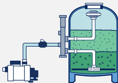
After installation, let AFM® soak to get it wet or run pool equipment on "filtration" for >24 hours to wet AFM®
