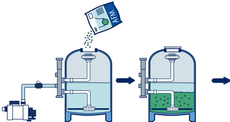
Fill up the filter with AFM® grades as determined in 1 and 2 above
