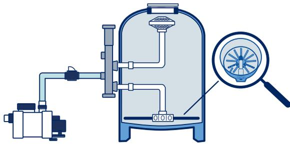
Before filling the filter with AFM®, check your filter's laterals and make sure they are not damaged.
