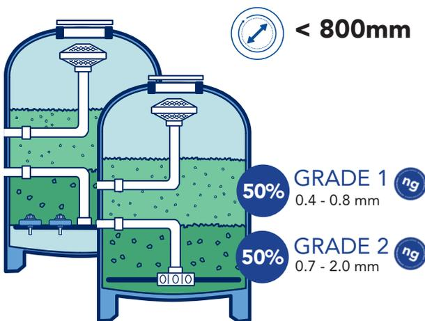
For smaller filters (< Ø 800 mm diameter) and for all filters with nozzle plate beds, irrespective of filter diameter: Use 50% of AFM® ng Grade 1 and 50% of AFM® ng Grade 2
