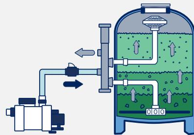
Proceed to first backwash >24 hours after installation at a velocity of 40 to 50 m/h ( $\text{m}^3/\text{h}/\text{m}^2$ )
