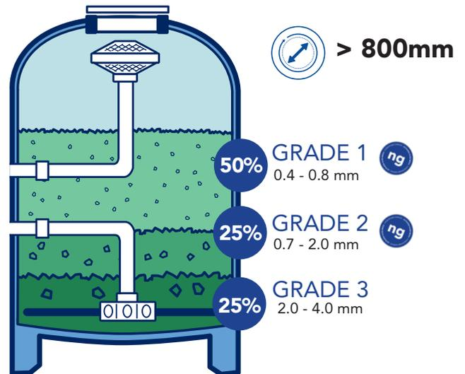
For larger diameter filters (> Ø 800mm) Use 50% of AFM® ng Grade 1, 25% of AFM® ng Grade 2 and 25% AFM® Grade 3. AFM® Grade 3 is required to cover big filter's laterals and, to ensure adequate water flow.
