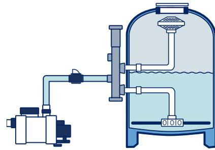
Half fill the filter with water to protect the laterals before pouring AFM® into the filter
